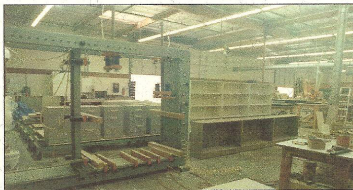
Cabinet assembly area with a pneumatic caseclamp
